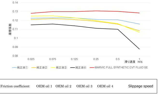
1. Results from the JASO M358 LFW-1 block on ring test (high load method)
